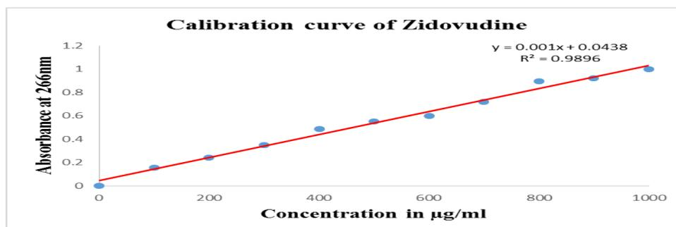
Figure 1: Standard Calibration Curve of Zidovudine in Phosphate buffer pH6.8
